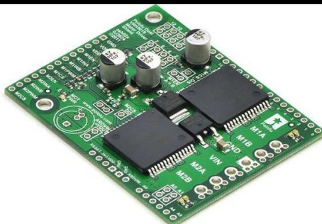
Figure 6: The Pololu Dual VNH5019 Motor Shield [Source: http://www.pololu.com/product/2502 ]
